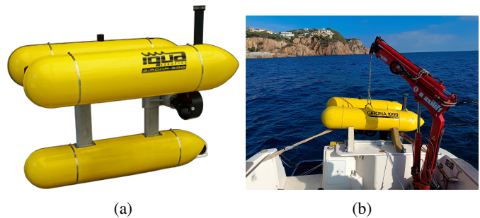
Fig. 2: Girona 1000 AUV: (a) general view and (b) robot deployment at sea using Sextant boat from Universitat de Girona.
